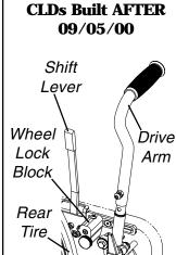
NOTE: Wheel lock block shown in vertical (wheel lock) position.
